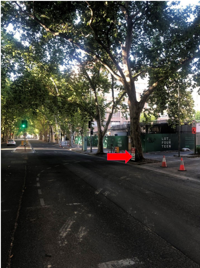
Poor visibility of pedestrian crossing for a vehicle waiting in right turn lane
